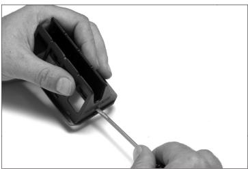
**Step 10**) Using a screwdriver or similar tool, push retainer bar flush with reed cage surface.
