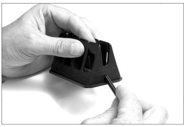
**Step 8)** Separate reeds and place new retaining bar (supplied) on an upward angle making sure it fits between the reeds.
