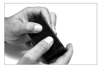
**Step 11**) Place reeds on outside surface and press on to locating tabs.
