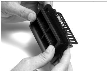
**Step 12**) With reeds in place, push reed cage through flange until locating tabs snap into their openings.
