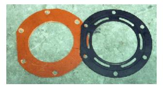
Make a gasket just like in the picture to block all of the water from flowing to the waterbox and use the OEM metal gasket as well on the waterbox side of the flange to reinforce it.
