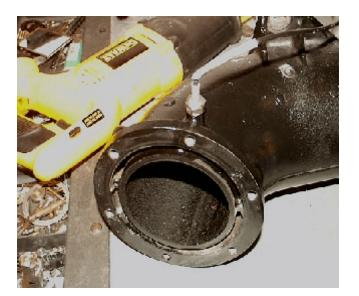
Install the OEM water temp sensor to the top 10mm tapped pipe nipple using Teflon tape.
