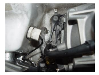
Remove your battery box and splice the siphon line that comes from the OEM bilge strainer
