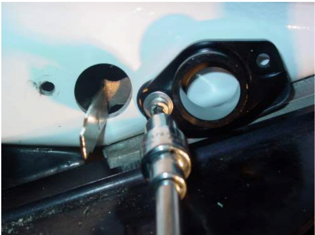
While holding the wrench with one hand I had assembled a allen socket on a nut driver handle and drove in slowly (It was a piece of cake)
