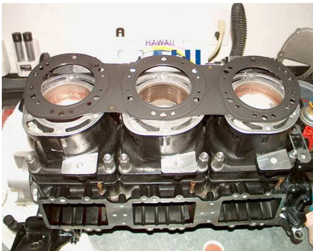
The head gasket only fits in one direction
