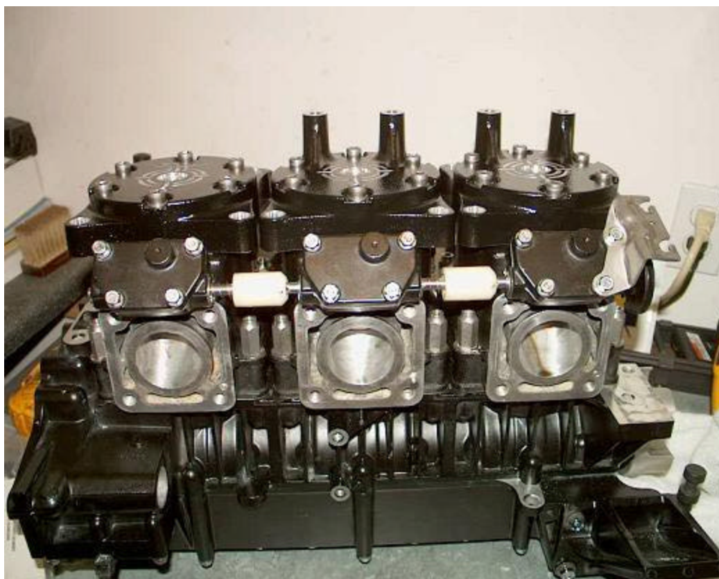
The head gasket only fits in one direction
