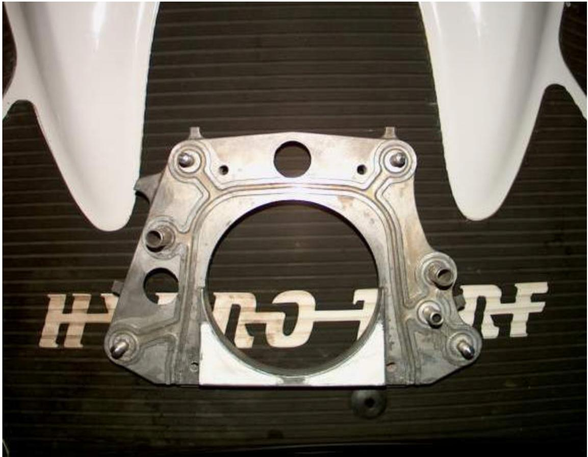
Seal triangular areas at the bottom of the transom plate with 3M5200 fast cure and let them cure for about 24 hours before you install the pump shoe
