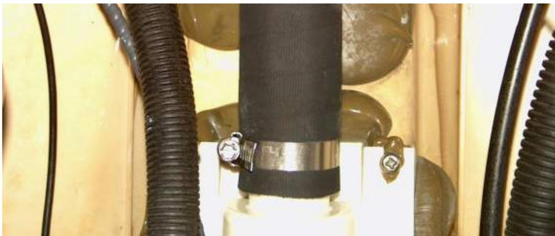
I replace the stock impeller shaft cover hose with a Gates brand which is vulcanized because my 99XLL OEM hose ruptured allowing the entire engine to flood being only 3 hours old. The cost of the hose is about \$8.00 to \$10.00 and you can pick one up at any Auto Parts store, just make sure that is not the one that has a wire coil inside.
