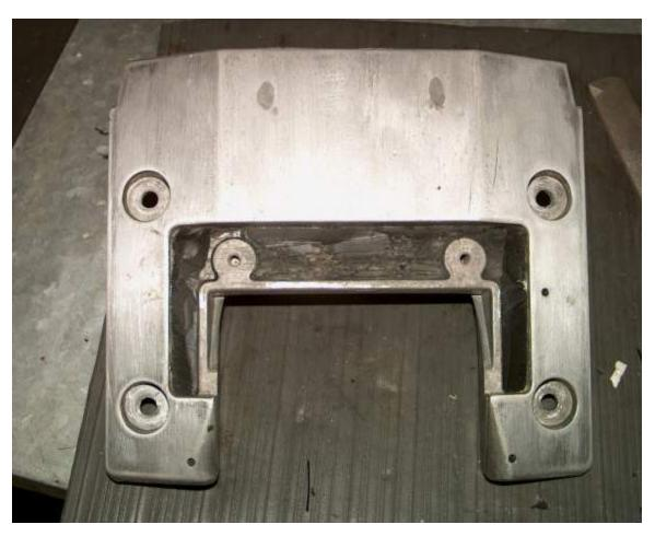
Remove some of the pump shoe material to allow the intake grate to be as flush as possible with the shoe. If not filing the top of the intake grate is recommended to math them up
